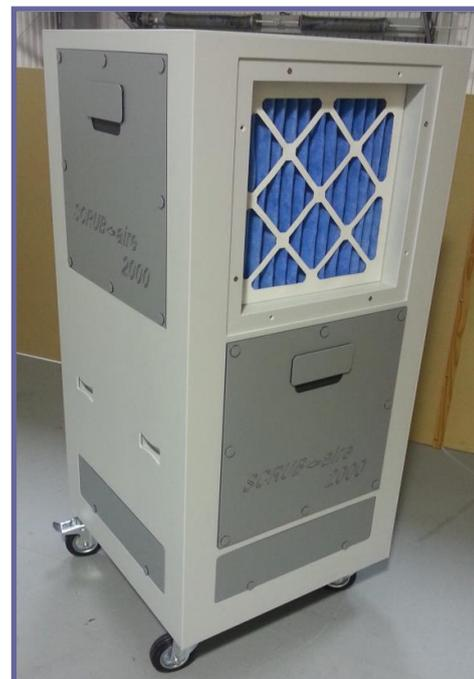
**General Specification:** the Scrub-aire 2000 has been designed to be easy to use, easy to clean, and provide air scrubbing duties within or close-by a work area. The Scrub-aire draws contaminated or polluted air through a series of filters, returning clean air at low level back to the work environment.
